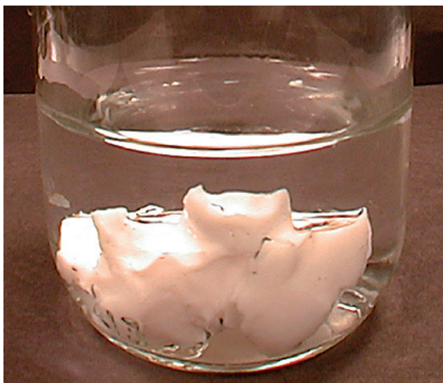
Krytox™ grease in hydrocarbon solvent is not dissolved.
