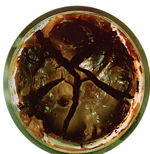
In oven at 232 °C (448 °F) for 40 hr: Hydrocarbon—40% wt loss
