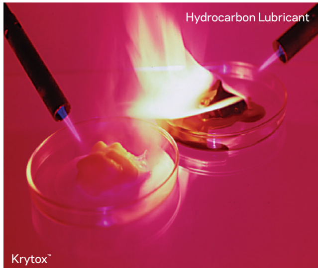
Hydrocarbon-based lubricants burn; Krytox™ does not.
